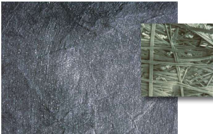
Figure 15. Non-woven heat bonded geotextile with close-up
