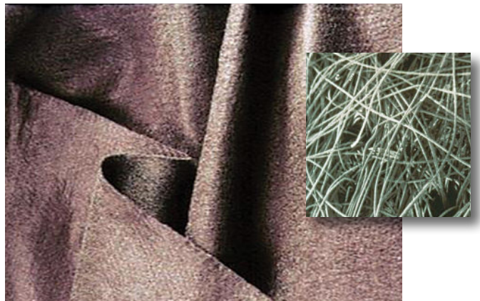
Figure 14. Non-woven needle punched geotextile with close-up
